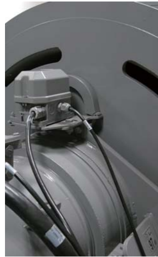
Upper and lower hoist limit switch
