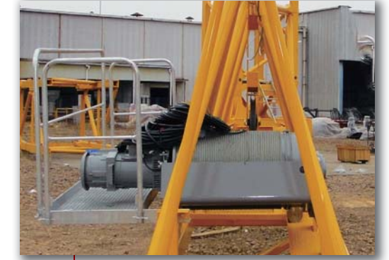
Platform giving access to the jib, allowing also to carry out the operations on the trolley winch and on the load limiter (settings are finished during commission)
