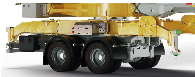
dual steering axle +20^{\circ}/-20^{\circ}
